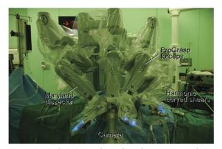
FIGURE 3. Single-incision robotic thyroidectomy; external view of robotic arms.
